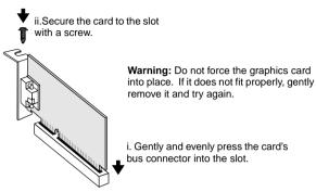
Figure 3: Securing the graphics card to the slot.
